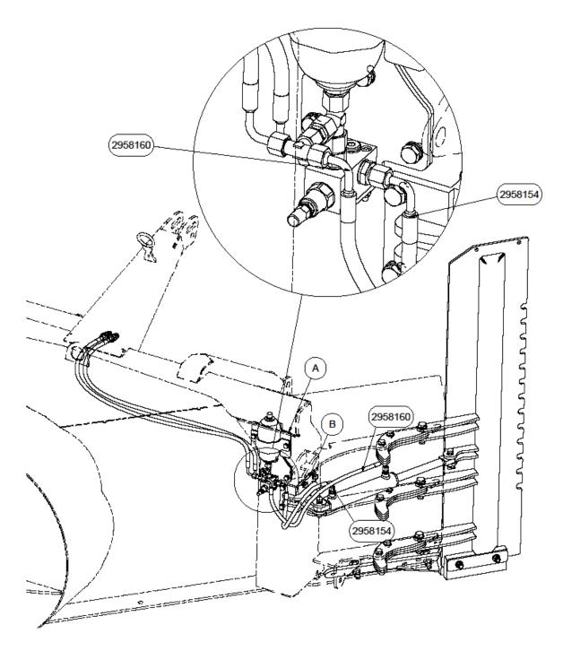
A: The bracket and plate for the accumulator must be assembled as in the illustration.
